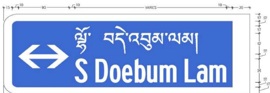
Figure 6.13. Standard street signage with a single street name & double headed arrow
