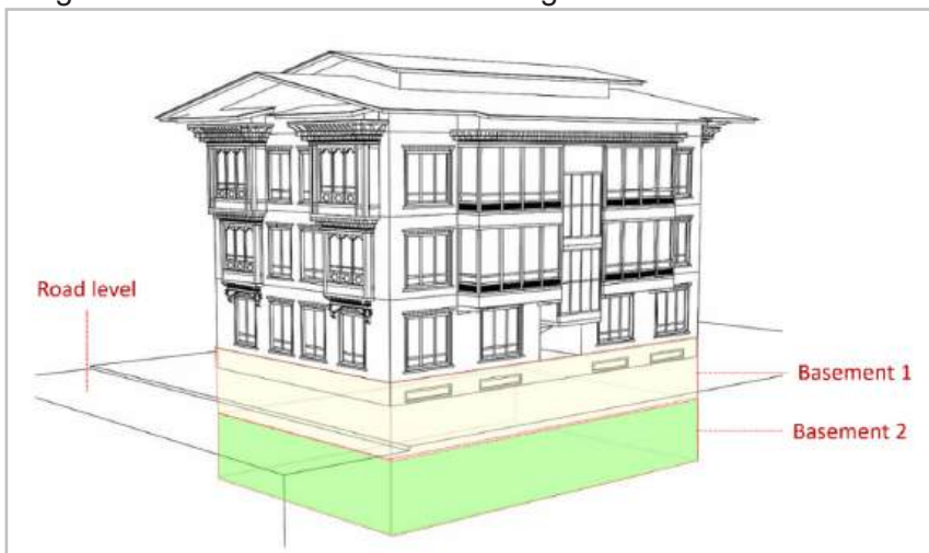
Figure 5.12. Floor levels of building with double basement
